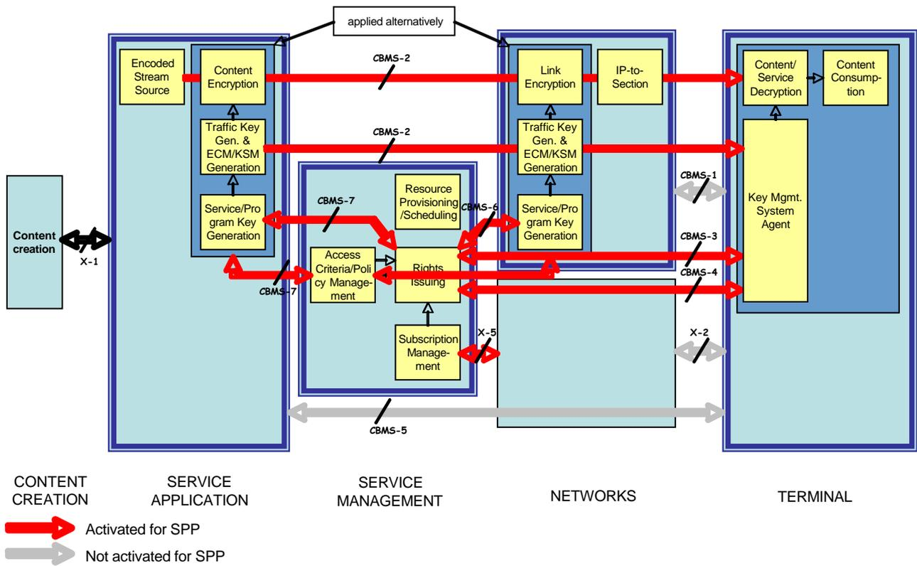
**Figure 14: Sub-Entities and reference points activated for Service Purchase and Protection**
