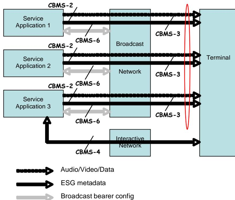
**Figure 5: Distributed ESG provisioning**
