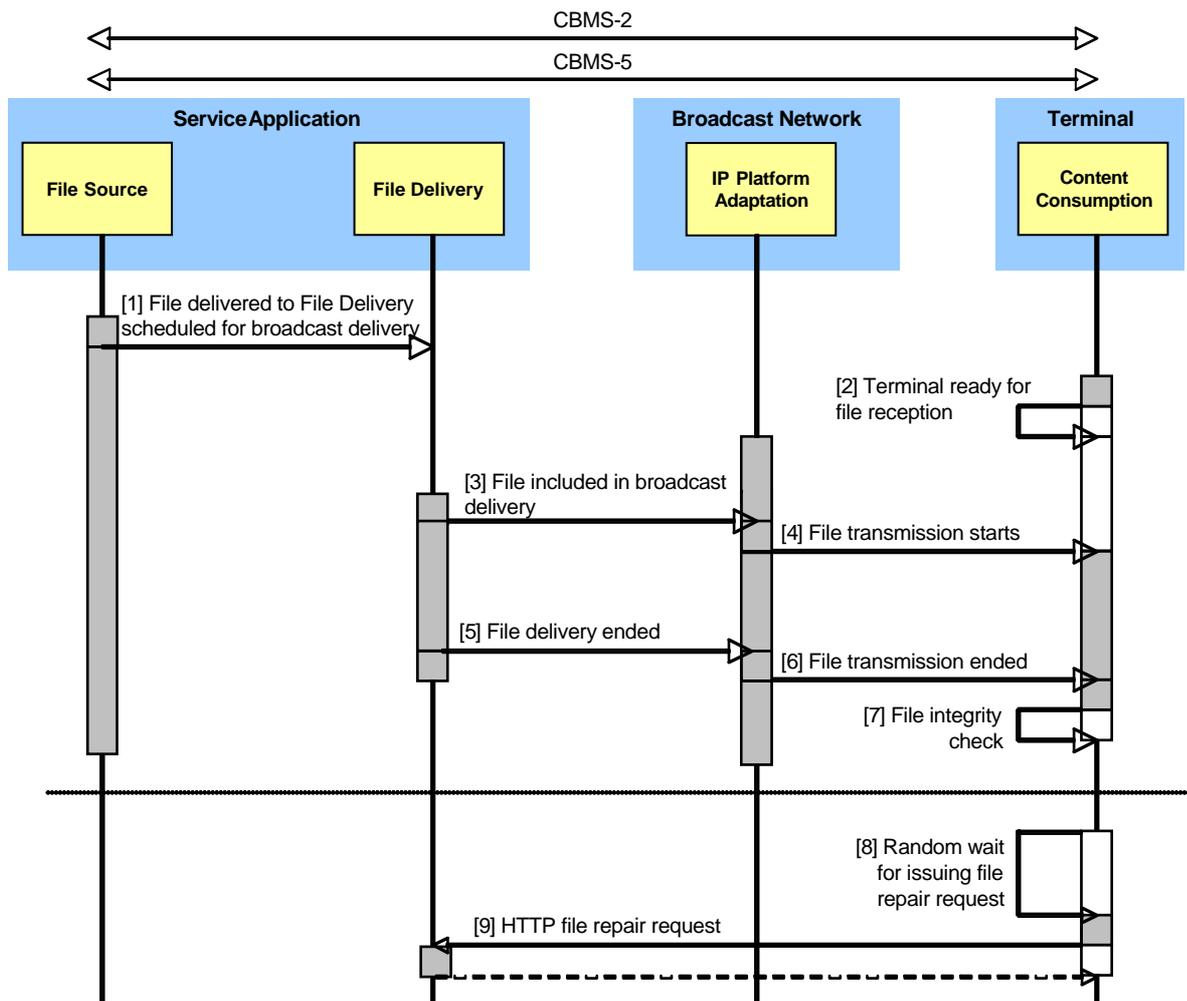
**Figure 12: Message flow for File Delivery**
