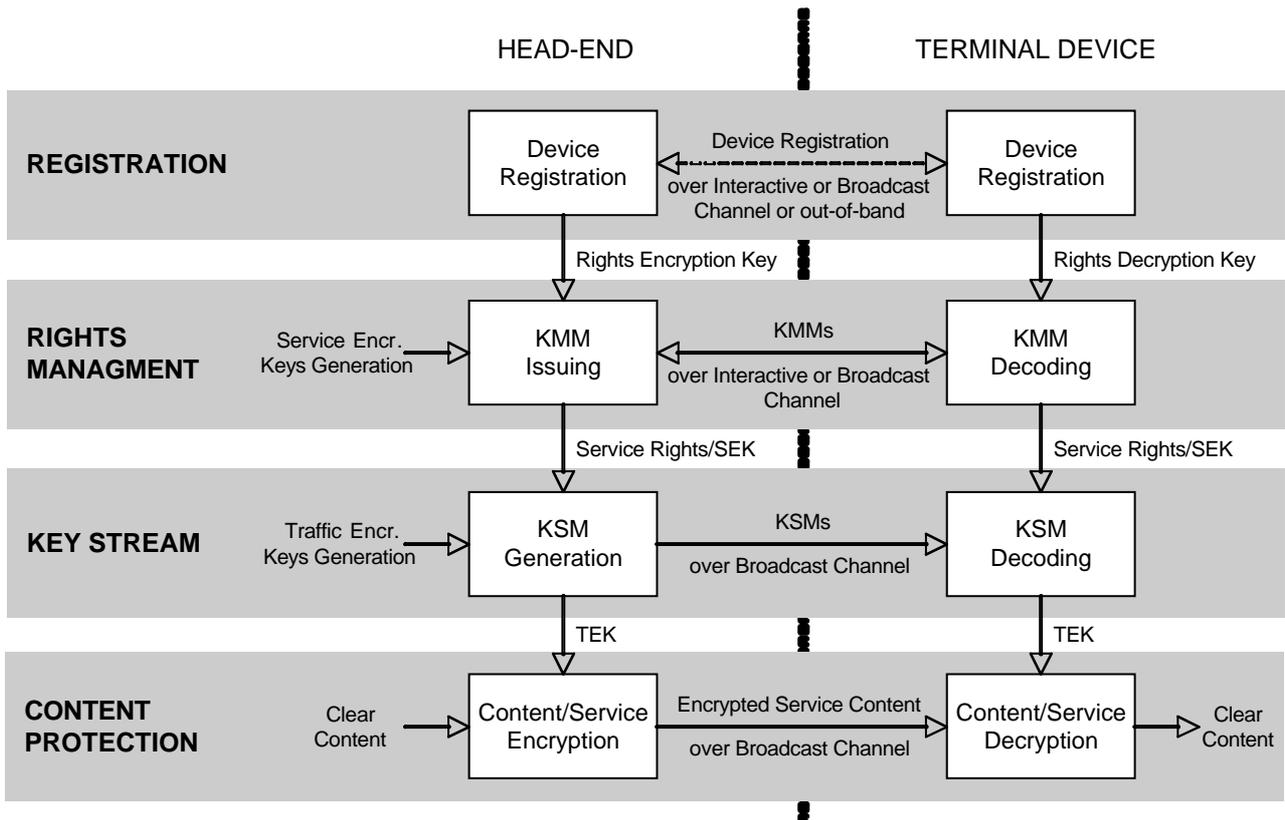
**Figure 13: Hierarchical Model for Service Protection**
