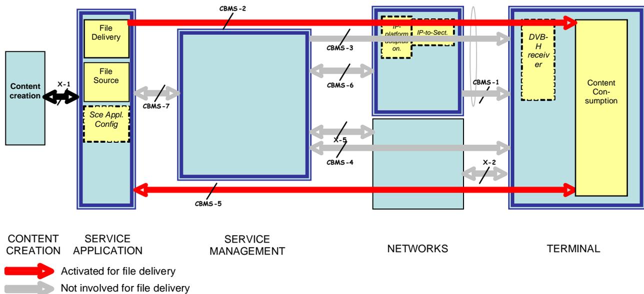
**Figure 11: Reference points activated for file delivery**
