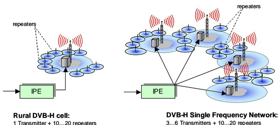
Figure 3: Possible network topology solutions for DVB-H
